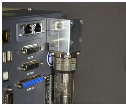
90° XCOM elbow connector
