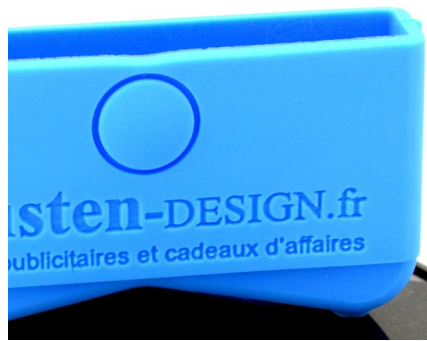
Non-contrasted marking on plastics
