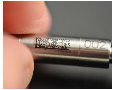
Annealing on stainless steel
